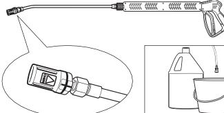
Step 1 To apply detergents the triple jet nozzle must be set to the "CHEM" position.
